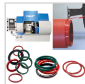
SKF Seal Jet system Customized Seals production
